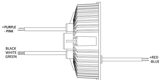
Maximum Wiring Distance (at full load) is 18AWG/18Feet
