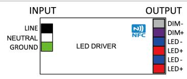
Maximum Wiring Distance (at full load) is 18AWG/18Feet LED case should be grounded
