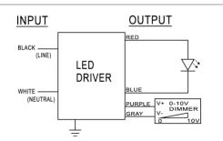
Maximum Wiring Distance (at full load) is 18AWG/18Feet LED case should be grounded
