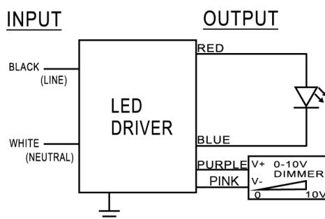
Maximum Wiring Distance (at full load) is 18AWG/18Feet
